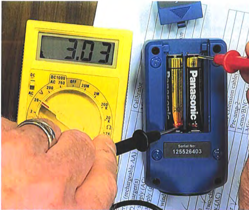
Fig. 6 Calibrator Battery Voltage, July 21
